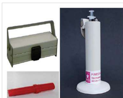
Figure 7: Different types of lead syringes for transporting radioactive material
